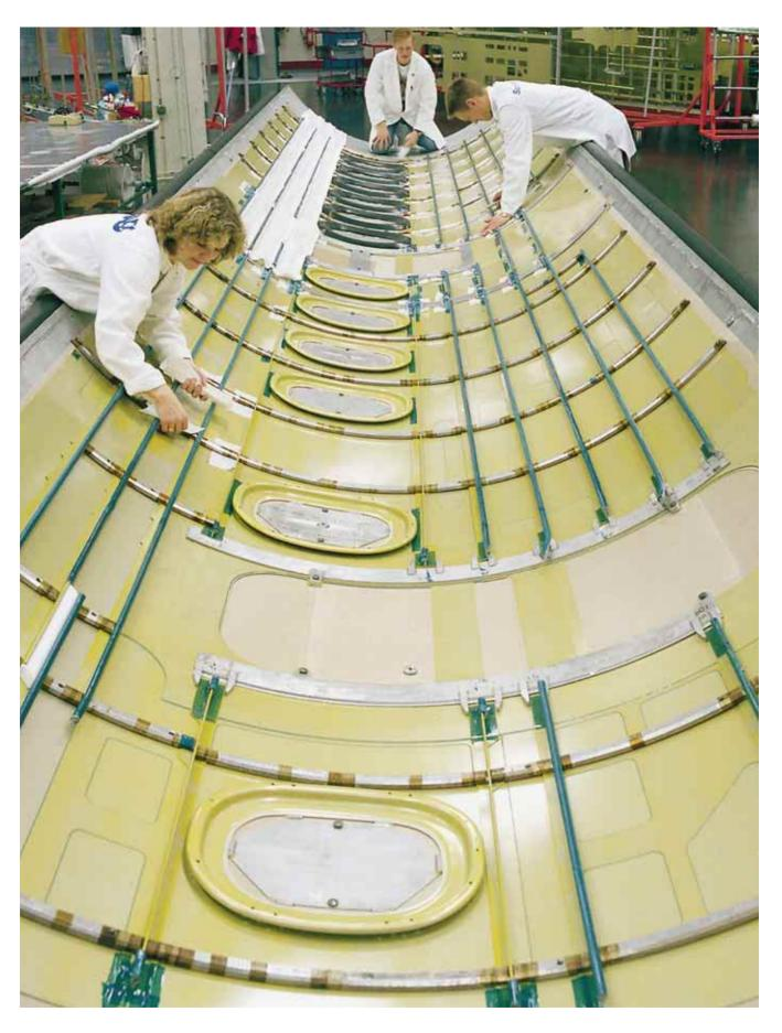
BONDING TOGETHER METAL PARTS INSTEAD OF USING TRADITIONAL RIVETING TECHNOLOGY, IS ONE OF SAAB'S SPECIAL EXPERTISE AREAS
