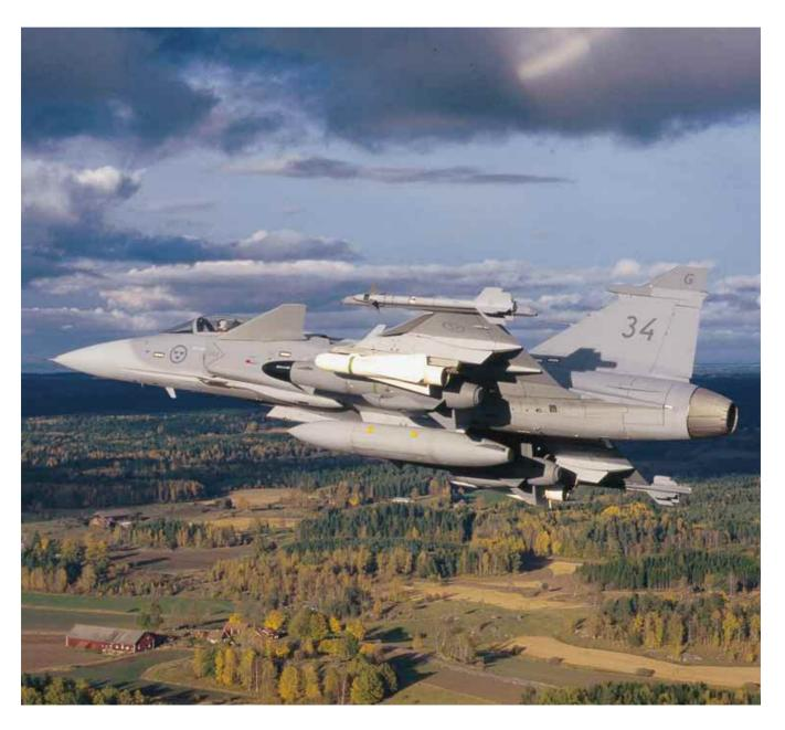
ONE OF THE APPROXIMATELY 50 AIRCRAFT NOW IN SERVICE WITH THE SWEDISH AIR FORCE, SEEN HERE WITH ATTACK ARMAMENT INCLUDING THE SAAB DYNAMICS RBS 15 MISSILE (WITH BLACK NOSE). THE AIRCRAFT IS PAINTED WITH A WATER-BASED PAINT INTRODUCED WITH BATCH 2, WHICH IS NOT ONLY MORE DISCREET BUT ALSO MORE ENVIRONMENT-FRIENDLY.
