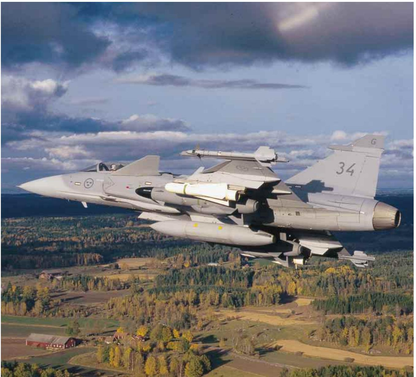
ONE OF THE APPROXIMATELY 50 AIRCRAFT NOW IN SERVICE WITH THE SWEDISH AIR FORCE, SEEN HERE WITH ATTACK ARMAMENT INCLUDING THE SAAB DYNAMICS RBS15 MISSILE (WITH BLACK NOSE). THE AIRCRAFT IS PAINTED WITH A WATER-BASED PAINT INTRODUCED WITH BATCH 2, WHICH IS NOT ONLY MORE DISCREET BUT ALSO MORE ENVIRONMENT-FRIENDLY.
